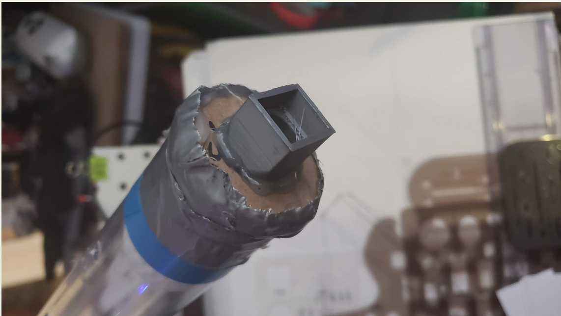
Figure 7. The outlet adapter at the base of the tube. [S1] Original image
